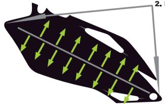
2. REMOVE PAPER LINER AND LINE UP TWO OPPOSITE CORNERS AND HOLES FIRST.
